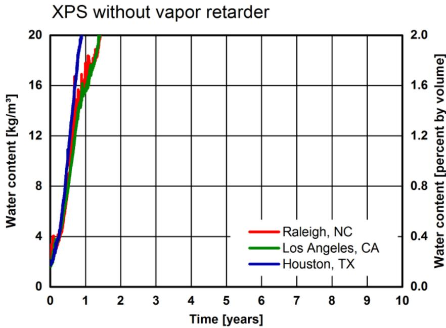
Figure 10. Insulation system: XPS without vapor retarder. Course of the water content over 10 years for Raleigh, Los Angeles, and Houston. For better comparison the scale is limited to 20 kg/m<sup>3</sup>; the whole course is displayed in Figure 8.
