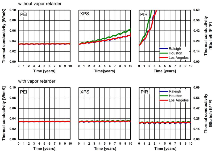
Figure 25. Thermal conductivity over 10 years for the three insulation systems without and with vapor retarder at all three locations (floating monthly mean values).
