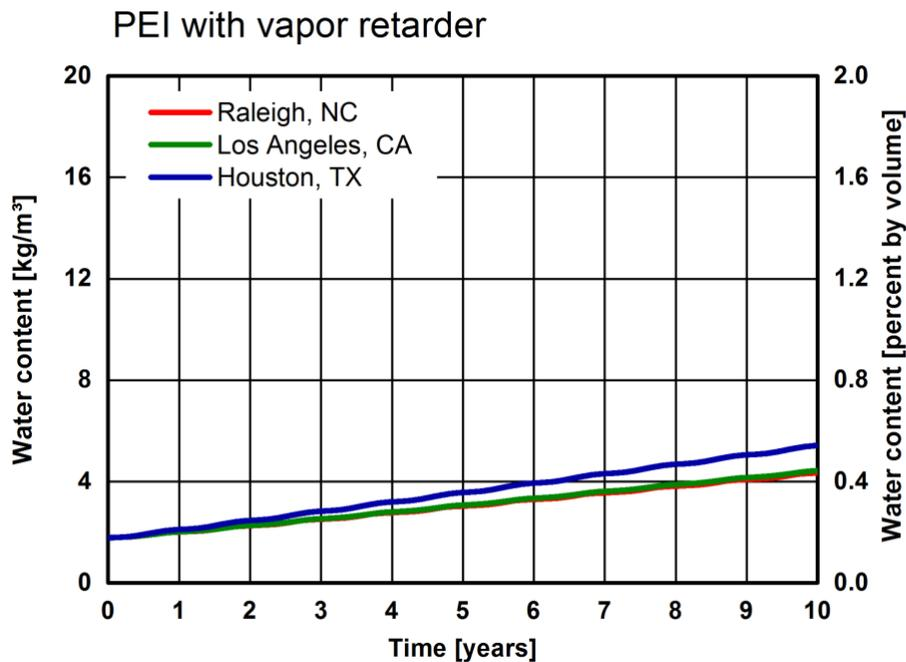
Figure 6. Insulation system: PEI with vapor retarder. Simulated total water content in the insulation layer over 10 years for Raleigh, Los Angeles, and Houston.
