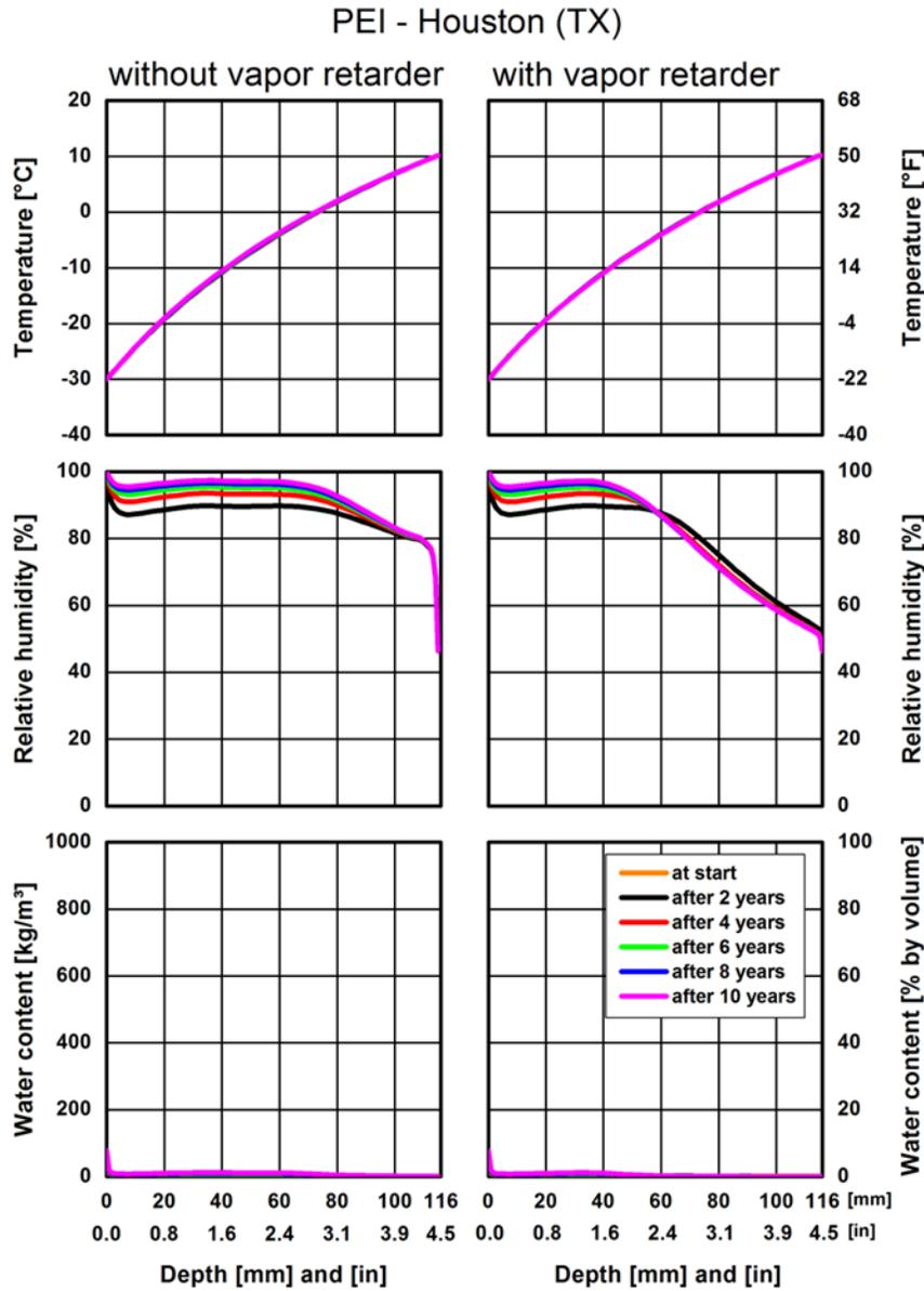
Figure 9. PEI, Houston (TX). Profiles for temperature, relative humidity, and water content after two, four, six, eight, and 10 years. The conditions at start are displayed for the water content only.
