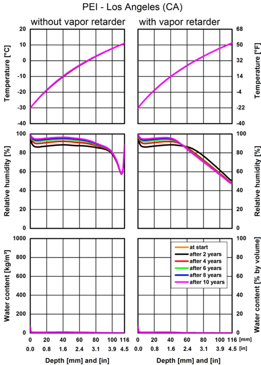
Figure 8. PEI, Los Angeles (CA). Profiles for temperature, relative humidity, and water content after two, four, six, eight, and 10 years. The conditions at start are displayed for the water content only.
