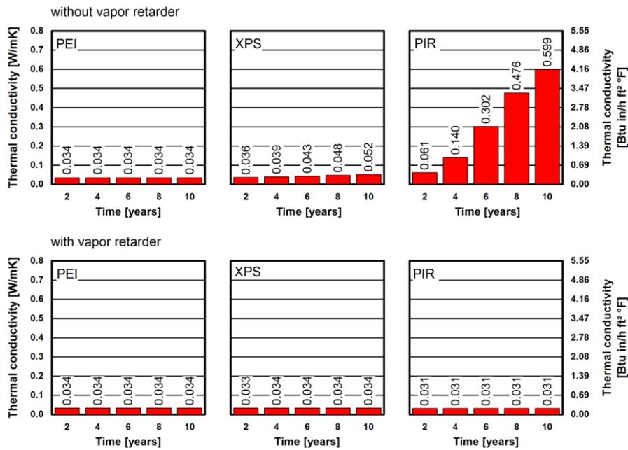
Figure 22. Raleigh (NC). Thermal conductivity of the three insulation systems without and with vapor retarder after two, four, six, eight, and 10 years.
