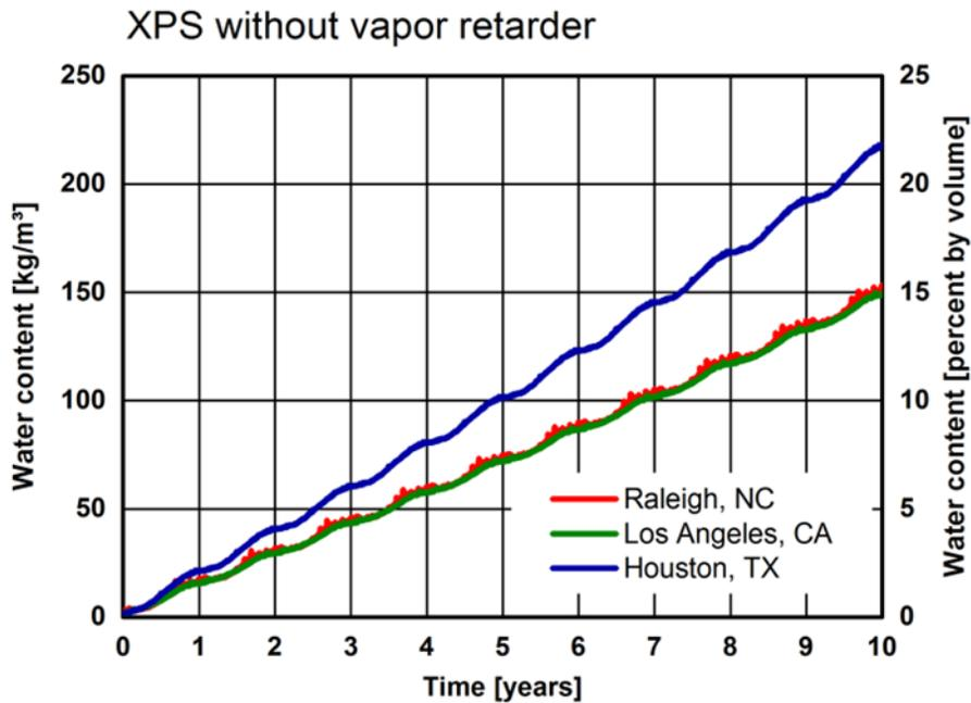
Figure 11. Insulation system: XPS without vapor retarder, complete course of Figure 7. Simulated total water content in the insulation layer over 10 years for Raleigh, Los Angeles, and Houston.
