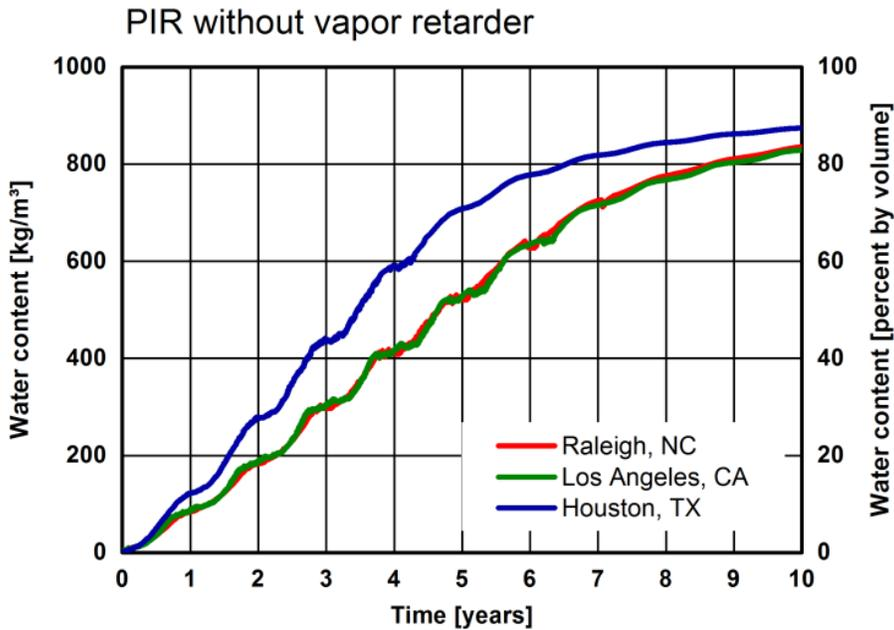
Figure 17. Insulation system: PIR without vapor retarder, complete course of Figure 10. Simulated total water content in the insulation layer over 10 years for Raleigh, Los Angeles, and Houston.
