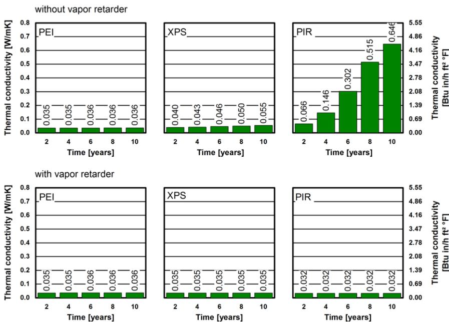
Figure 23. Los Angeles (CA). Thermal conductivity of the three insulation systems without and with vapor retarder after two, four, six, eight, and 10 years.
