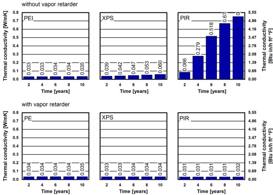
Figure 24. Houston (TX). Thermal conductivity of the three insulation systems without and with vapor retarder after two, four, six, eight, and 10 years.
