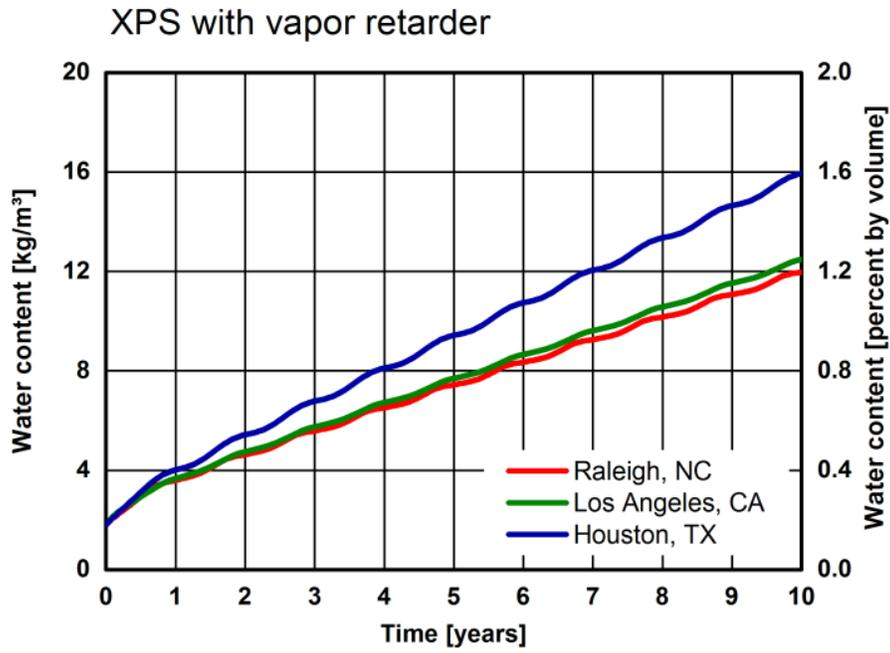
Figure 12. Insulation system: XPS with vapor retarder. Simulated total water content in the insulation layer over 10 years for Raleigh, Los Angeles, and Houston.
