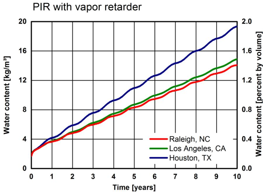
Figure 18. Insulation system: PIR with vapor retarder. Simulated total water content in the insulation layer over 10 years for Raleigh, Los Angeles, and Houston.
