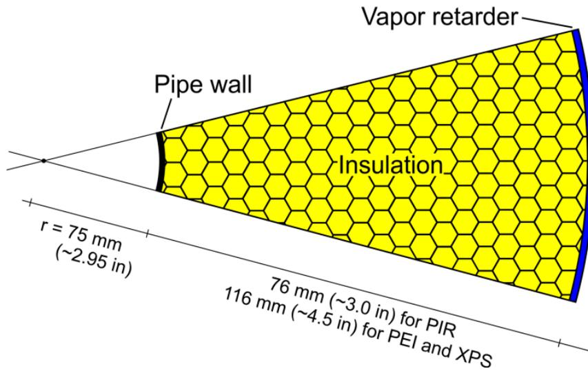
Figure 1. Schematic drawing of a cross section of the pipe insulation system.
