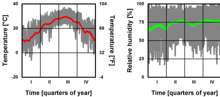
Figure 4. Temperature and relative humidity for Houston, TX. The gray area shows hourly values, the colored line the flowing monthly mean value.
