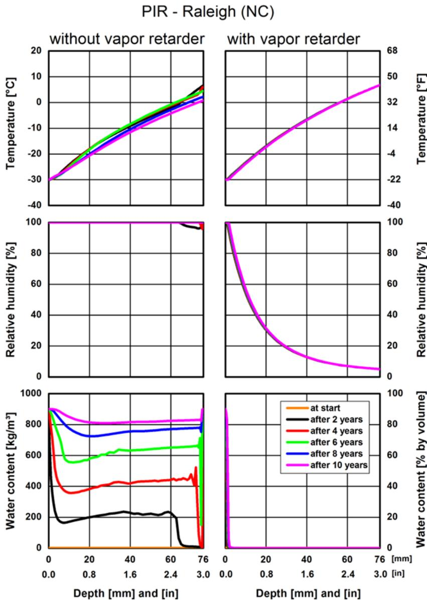
Figure 19. PIR, Raleigh (NC). Profiles for temperature, relative humidity, and water content after two, four, six, eight, and 10 years. The conditions at start are displayed for the water content only.
