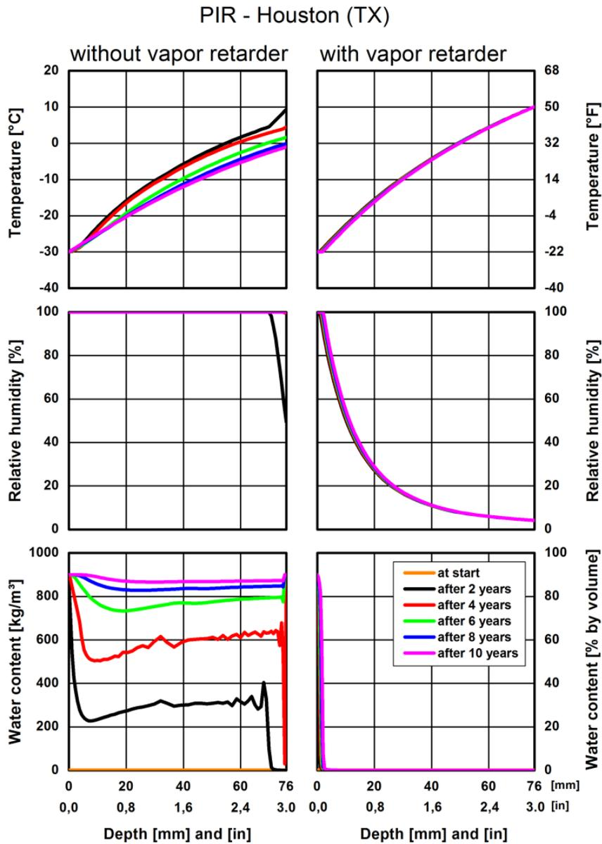
Figure 21. PIR, Houston (TX). Profiles for temperature, relative humidity, and water content after two, four, six, eight, and 10 years. The conditions at start are displayed for the water content only.
