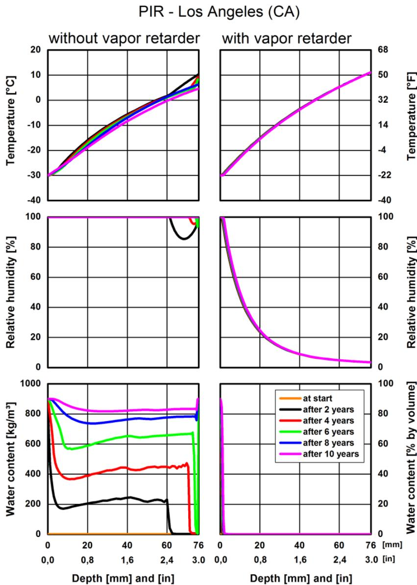
Figure 20. PIR, Los Angeles (CA). Profiles for temperature, relative humidity, and water content after two, four, six, eight, and ten years. The conditions at start are displayed for the water content only.
