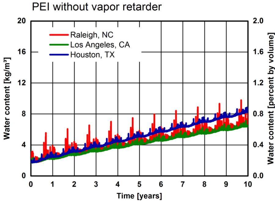
Figure 5. Insulation system: PEI without vapor retarder. Simulated total water content in the insulation layer over 10 years for Raleigh, Los Angeles, and Houston.
