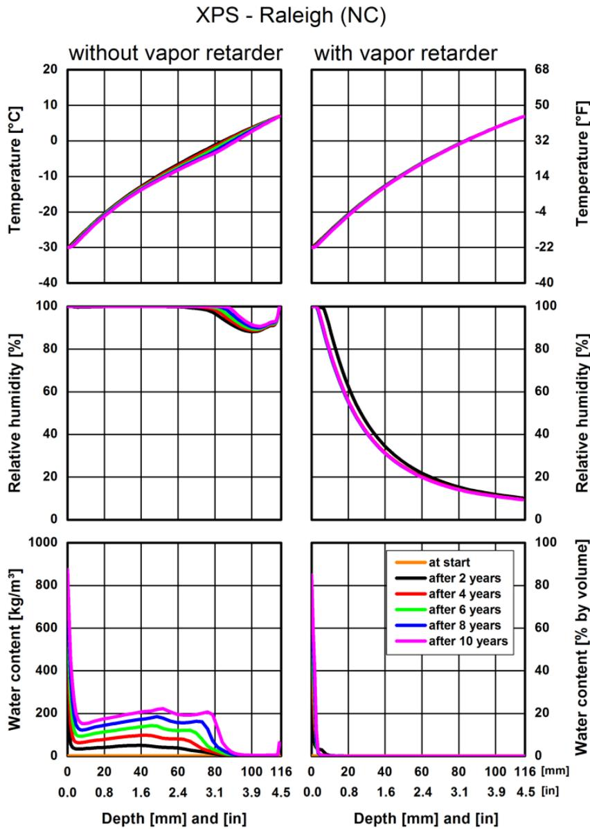
Figure 13. XPS, Raleigh (NC). Profiles for temperature, relative humidity, and water content after two, four, six, eight, and ten years. The conditions at start are displayed for the water content only.
