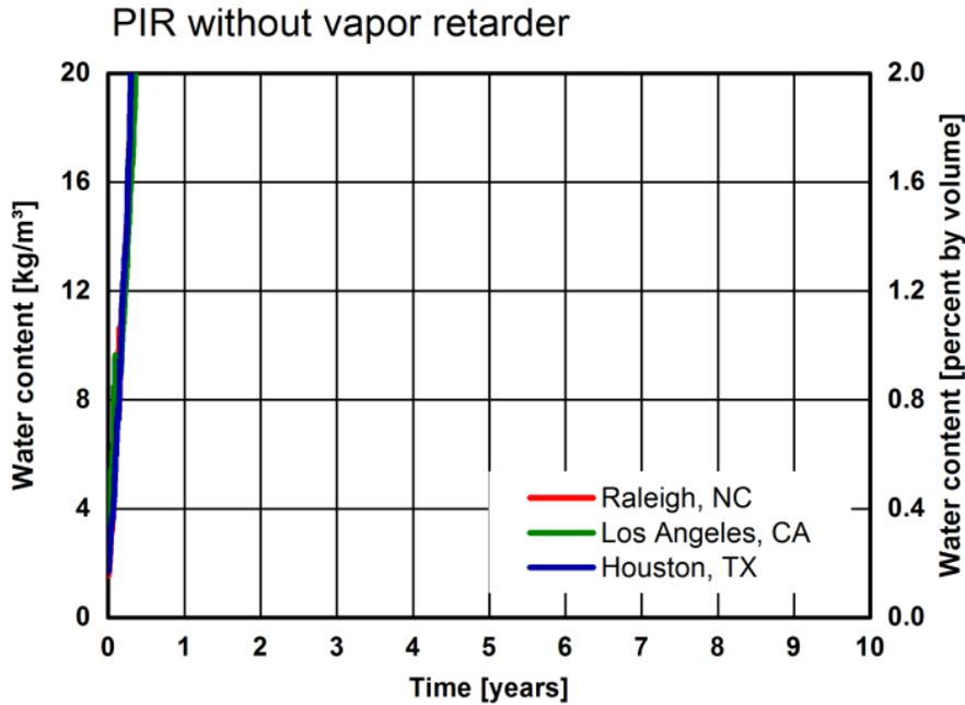
Figure 16. Insulation system: PIR without vapor retarder. Course of the water content over 10 years for Raleigh, Los Angeles, and Houston. For better comparison the scale is limited to 20 kg/m<sup>3</sup>; the whole course is displayed in Figure 11.
