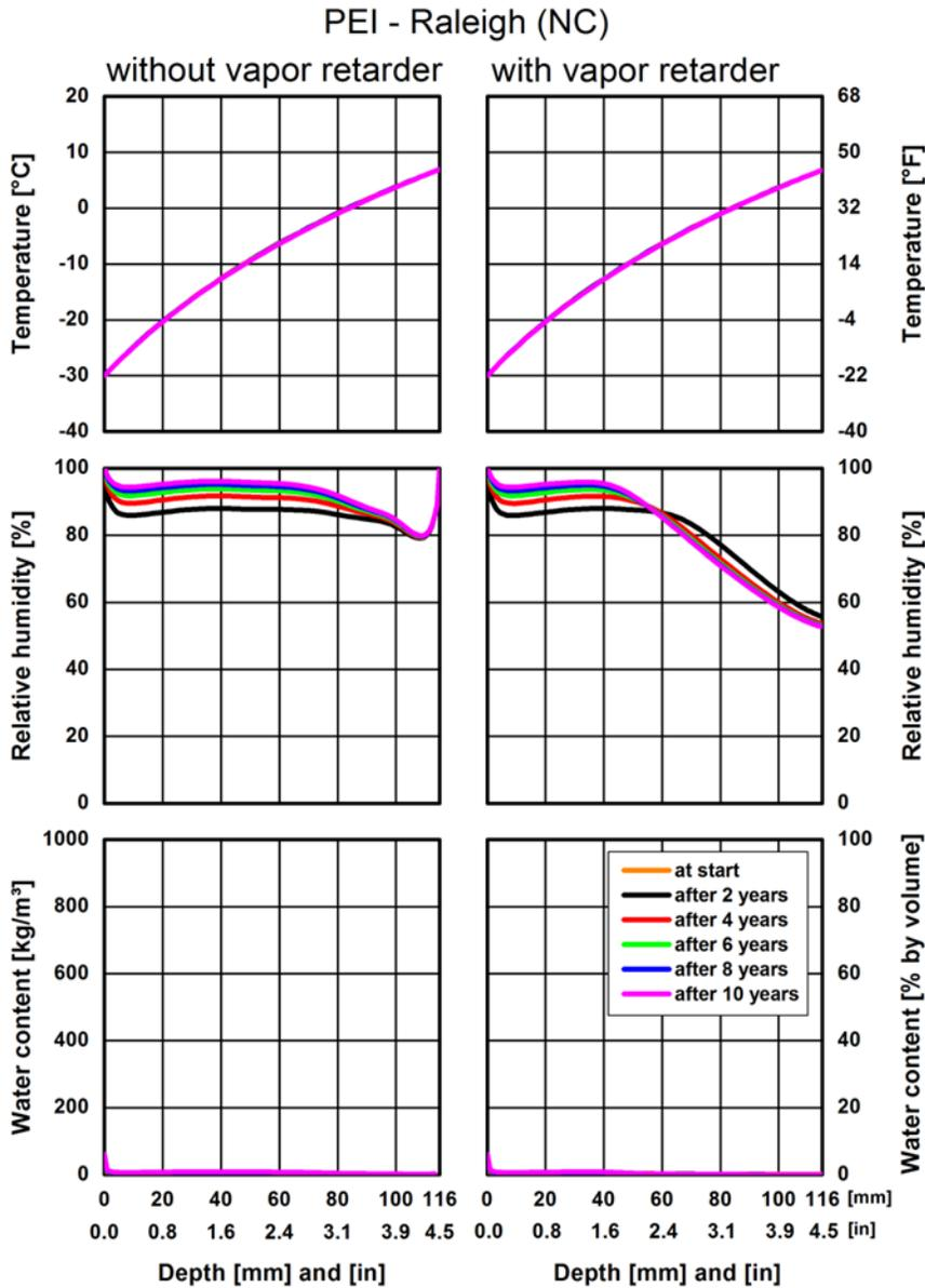
Figure 7. PEI, Raleigh (NC). Profiles for temperature, relative humidity, and water content after two, four, six, eight, and 10 years. The conditions at start are displayed for the water content only
