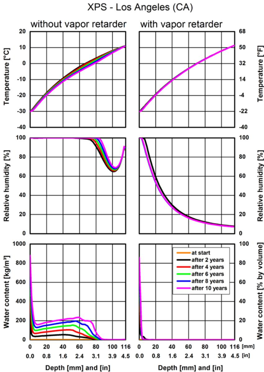
Figure 14. XPS, Los Angeles (CA). Profiles for temperature, relative humidity, and water content after two, four, six, eight, and ten years. The conditions at start are displayed for the water content only.
