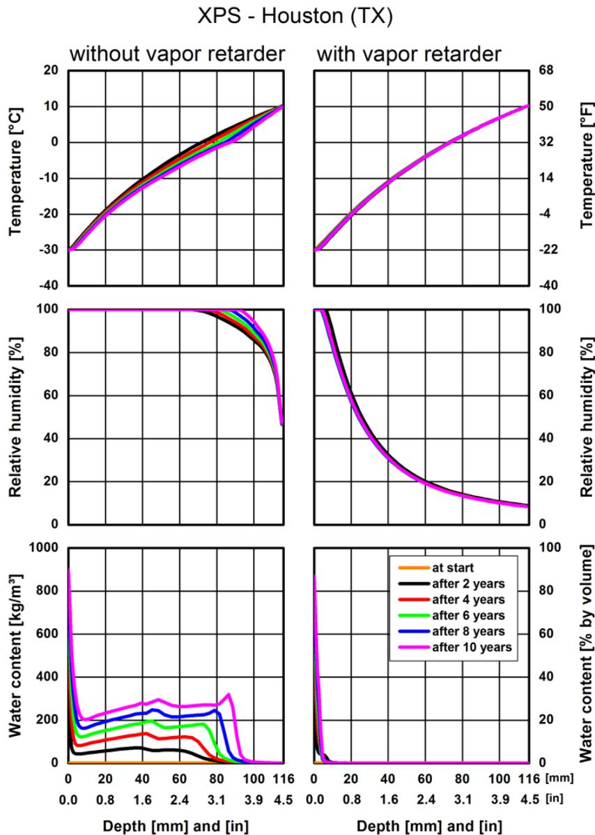
Figure 15. XPS, Houston (TX). Profiles for temperature, relative humidity, and water content after two, four, six, eight, and ten years. The conditions at start are only displayed for the water content.
